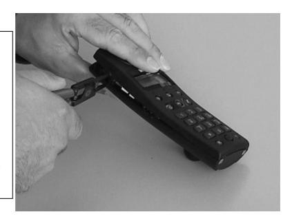
Insert pliers between the case shells near the display and press pliers together until remaining snap hooks open.
