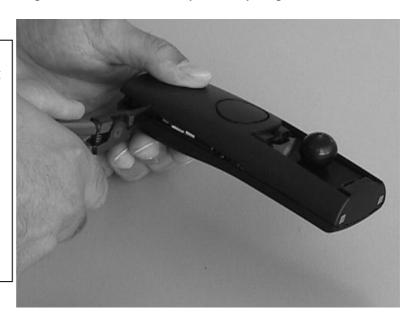
Turn handset upside down and insert pliers in the 2. belt clip hole and press pliers together until snap hooks open.
