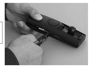
Make sure that the battery dummy is still fixed and lift off lower case shell as described in the picture. Hold the board with the other hand while lifting the case shell. Make sure that you don't bend the battery contact springs!
