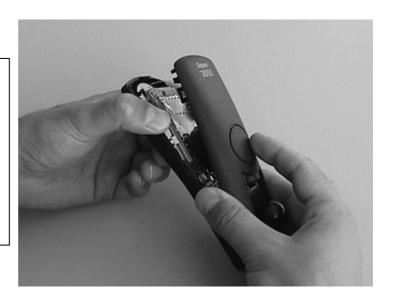
Use pliers to take out the charger contact springs. Take out the board.
