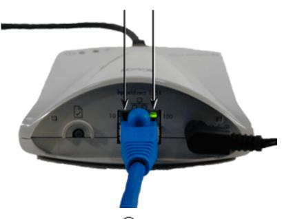
• The power/status LED ① on the top front begins blinking and within 15 seconds is solid green, to indicate the server passed its self test.
