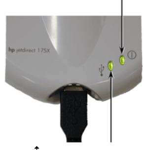
• The USB LED  $\stackrel{•}{\Psi}$  on the top front indicates the USB-II connection status. See above.
