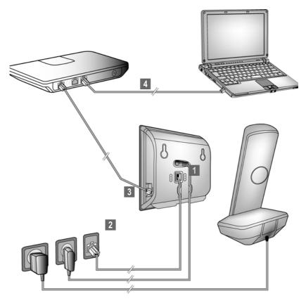
Bild 1 Connecting the phone to the fixed line network and the Internet
