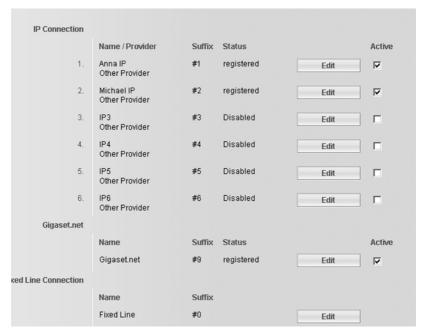
Bild 2 List of possible connections
